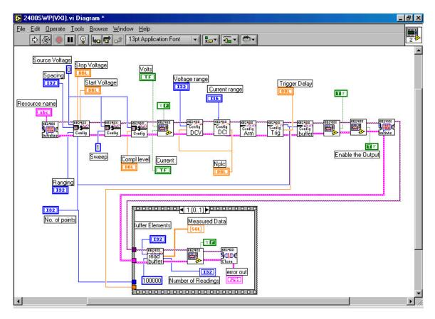
This is a complete and working example done in LabVIEW 6. It makes use of the VXI/PnP driver for SourceMeter Instruments. The defaults of the example perform a voltage sweep from 0V to 5V in 13 steps. The measured data (in amperes) is then displayed. If the example does not exactly fit your application then it can be used as a model to build upon to achieve the desired performance.
